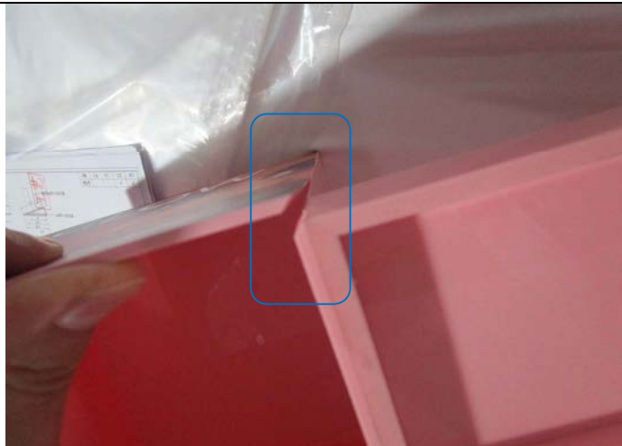
The artwork box panel is loosed (the glue is not firmly attached)
