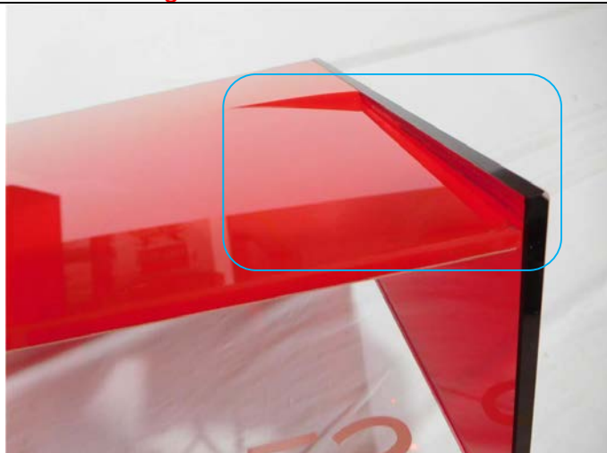
The window is cracked (the glue is not firmly attached).
