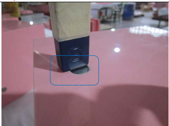
The magnet is not magnetized
